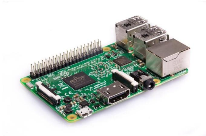
Figura 2 - Placa Raspberry Pi 3 Model B<sup>3</sup>
