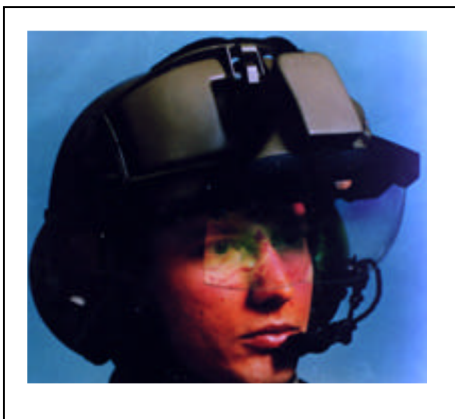
Figura 1. Capacete Optical See-Through HMD (Fonte: AZUMA, 1997)
